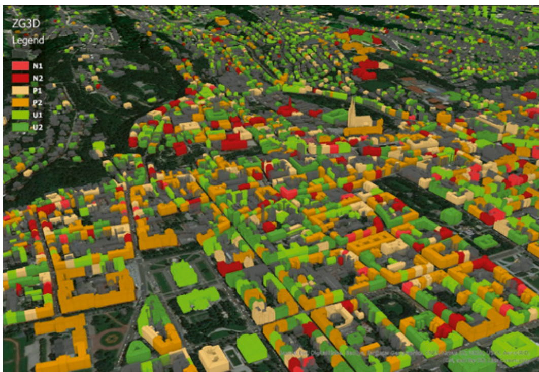
Source: University of Zagreb Faculty of Civil Engineering. Notes: 3D model of buildings represented by the usability classifications color (green, yellow, and red).
